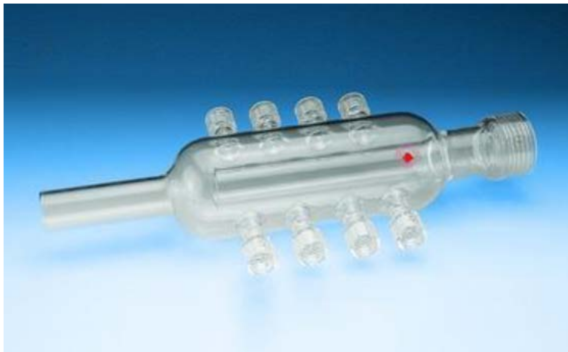
Figure 3-3. Photo of an 8-Port CARB Octopus Sample Manifold
