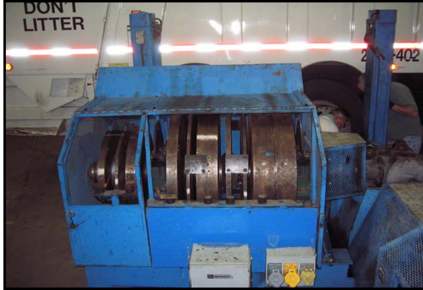
Figure 2: Flywheels were used to simulate vehicle inertia.
