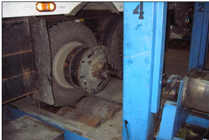
Figure 1: Hub adapters connect the vehicle's drive axle to the power absorber unit.
