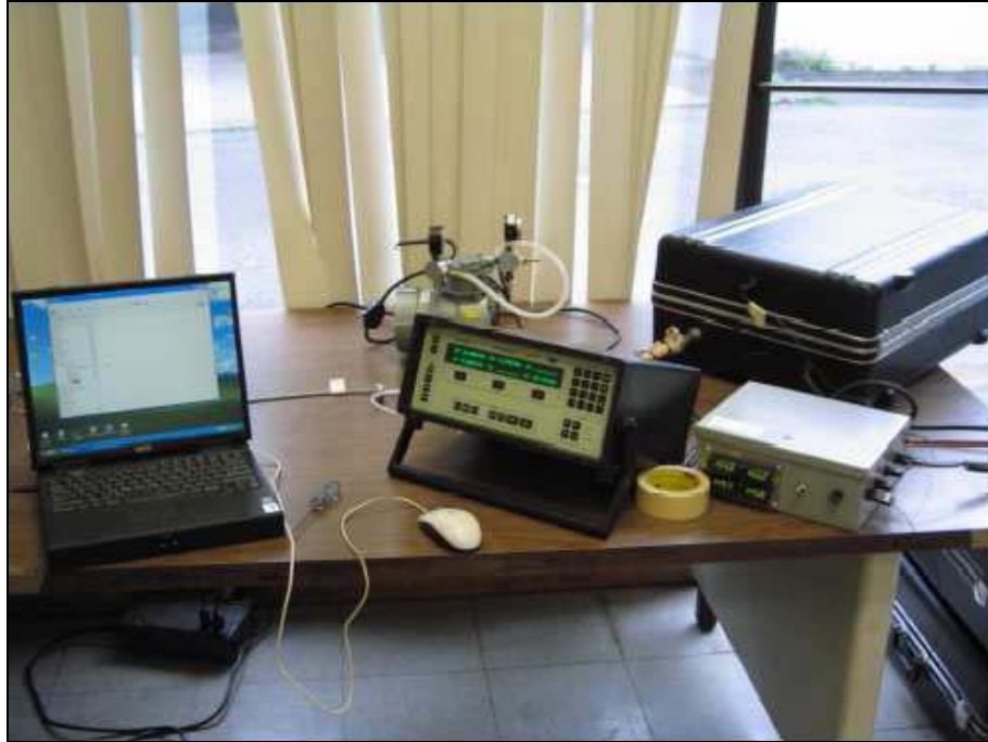
Figure 4: Innova 1302 Photoacoustic analyzer and sampling system.
