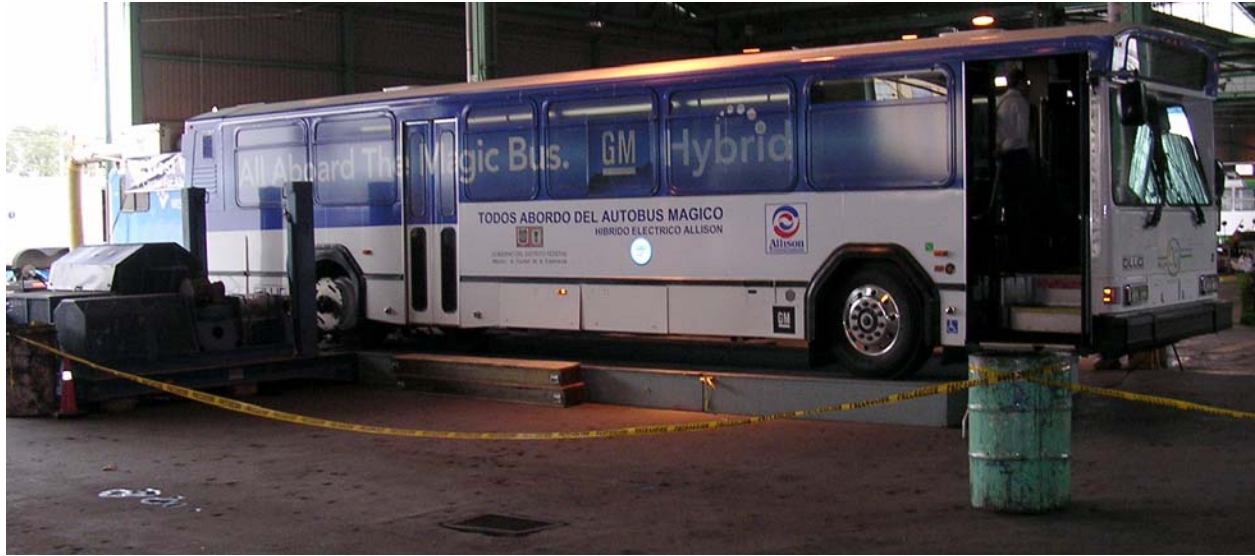
Figure 3: WVU Transportable Laboratory testing the Allison hybrid-electric bus.
