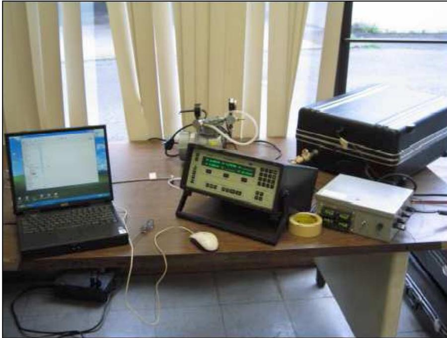
Figure 4: Innova 1302 Photoacoustic analyzer and sampling system.
