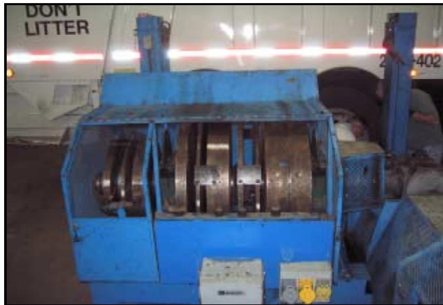
Figure 2: Flywheels were used to simulate vehicle inertia
